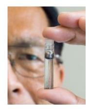
Test tube full of Hitachi 'RFID powder' (Mu chip) 0.05 x 0.05 mm.
